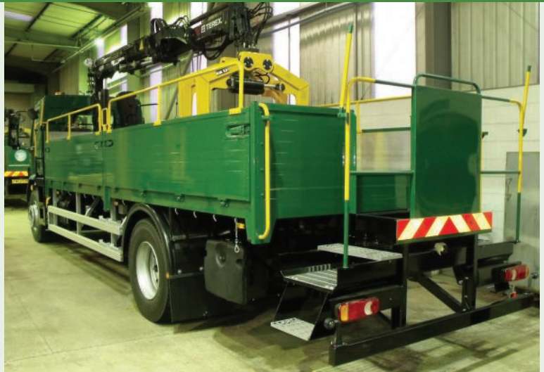
Above: Travis Perkins access step with grab handles. Developed in 2009 and fitted at the rear of all two-axle delivery trucks with front-mounted cranes
